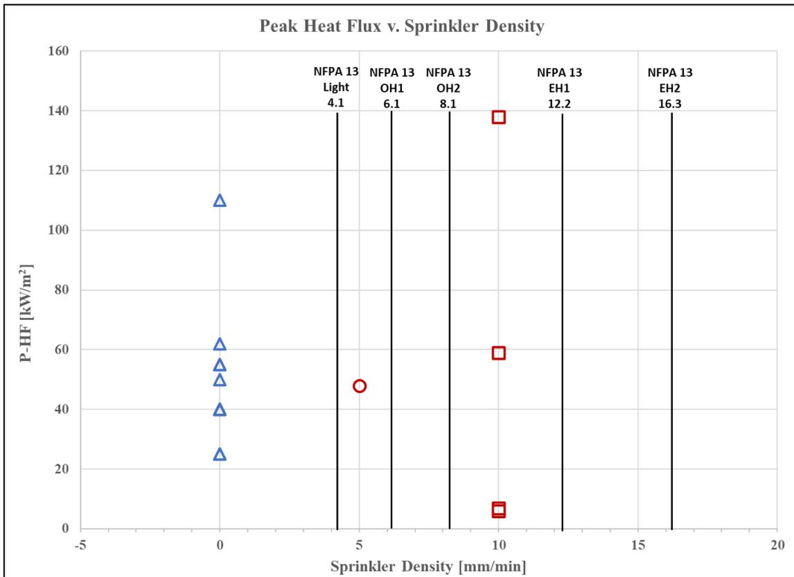
Figure 39. Peak heat flux at the neighboring vehicle location in testing documented in the literature database as a function of the sprinkler density. Blue triangles represent vehicle fire tests with no sprinklers, red circles represent tests with a sprinkler density of 5 mm/min and red squares represent tests with a sprinkler density of 10mm/min.
