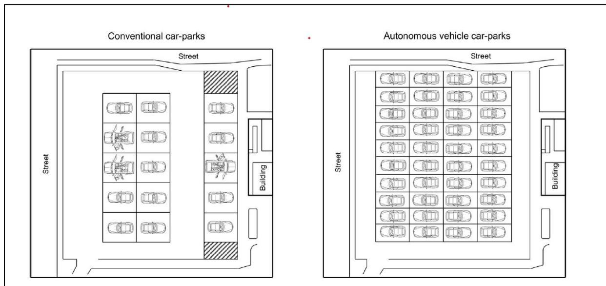
Figure 6. Potential differences between conventional parking garages (car-parks) and autonomous vehicle parking garages (car-parks) (reproduced from [9]).
