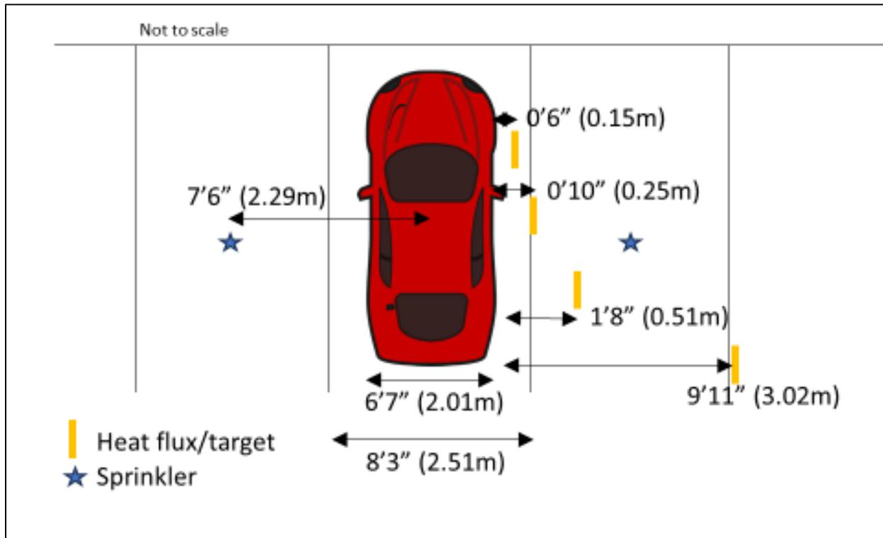
Figure 40. Proposed reasonably feasible test layout of sprinklers and heat flux targets.
