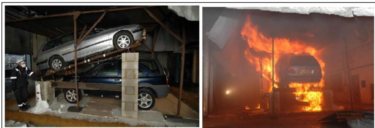
Figure 36: Test 11 as published in BRE report [18]. First image (left) shows the setup of the stacker test. The second image (right) shown is 10 minutes and 10 seconds after the fire was started at driver side seat of the bottom car with the windows open.
