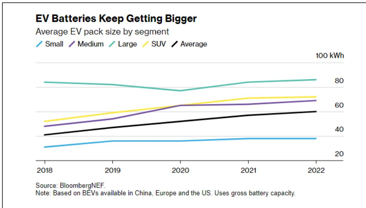
Figure 11. EV battery capacities as a function of time (source: Bloomberg).
