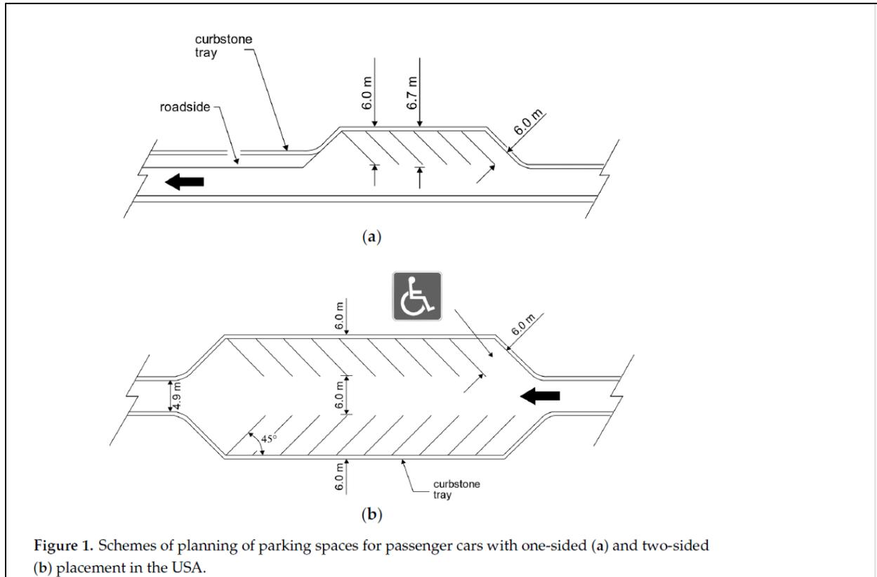
Figure 1. Schemes of planning of parking spaces for passenger cars with one-sided (a) and two-sided (b) placement in the USA [3].
