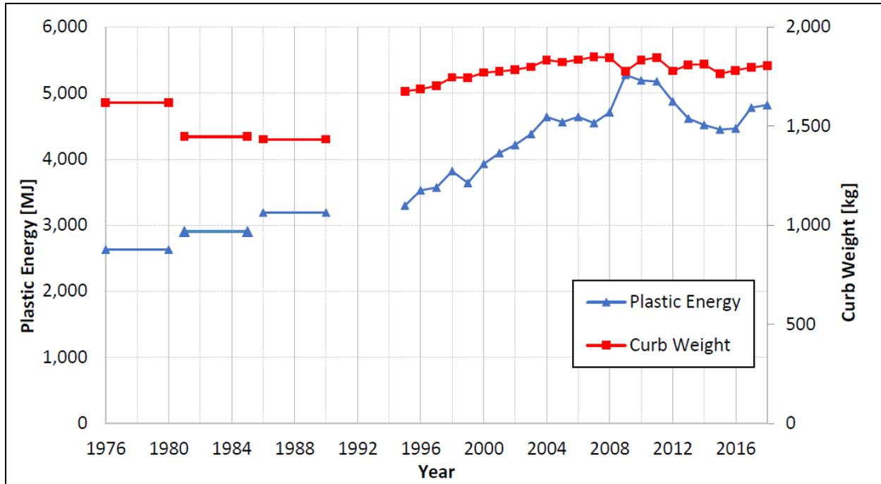
Figure 8. Calculated plastic energy and vehicle curb weight as a function of time (Figure 6 from [1]).
