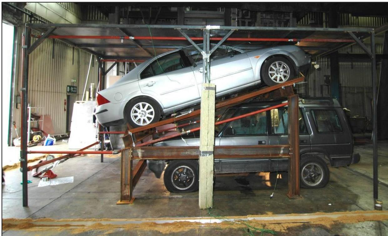
Figure 37: BRE [61] (Figure 3 in the publication) test setup for the stacker vehicle fire test with sprinklers. Eight automatic sprinkler heads (60°C) were installed, one near every corner of each vehicle.
