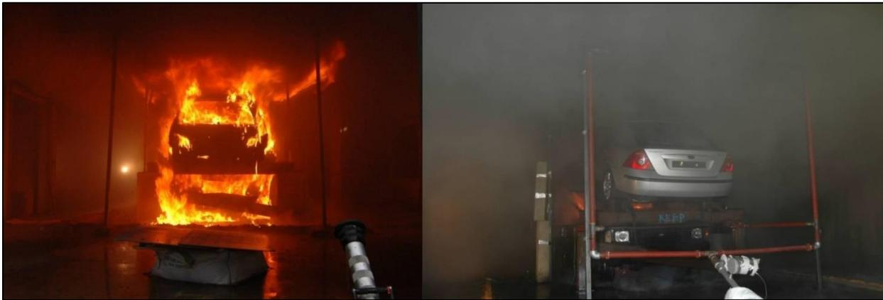
Figure 38: The stacker test images shown are at about 21 minutes after the start of the fire at the bottom vehicle driver side seat for both tests as performed by BRE [18] [61], no sprinklers (left) and with sprinklers (right). (Images taken from Figures 27 and 28 of BRE [61]). The sprinklers activated (right image) starting at about 13 minutes after the start of the fire.
