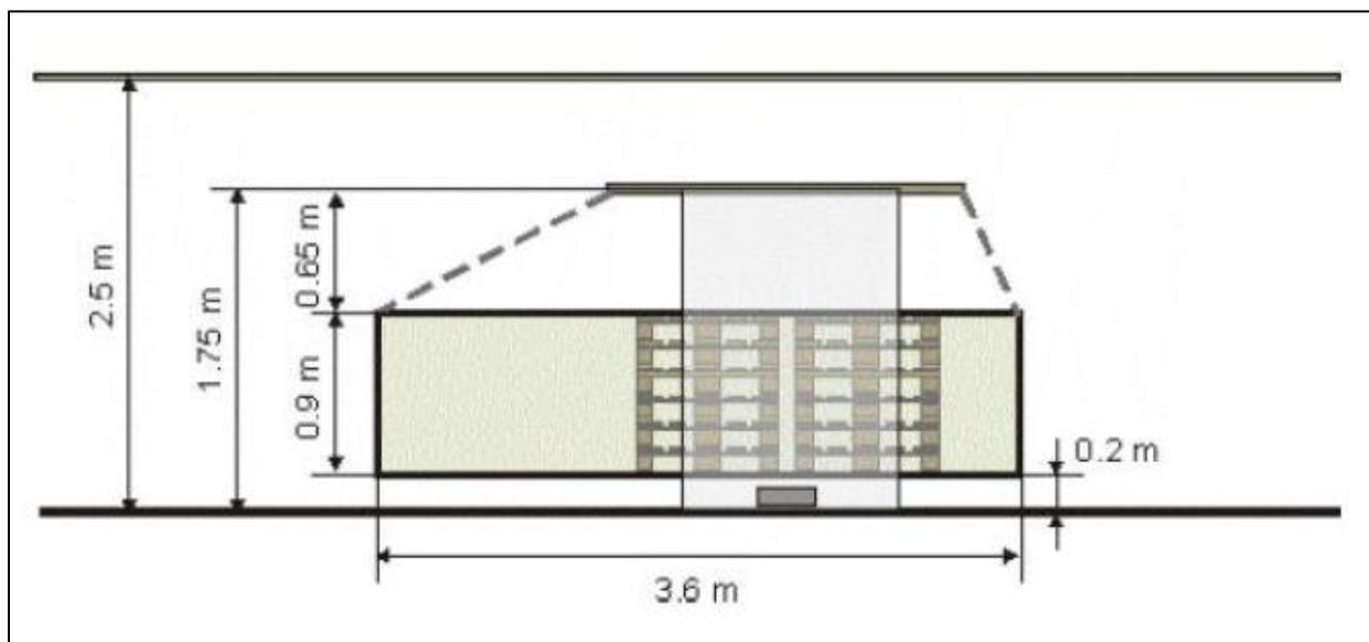
Figure 41. Side view of the standardized mock-up passenger vehicle fire source utilized in the IMO ro-ro vessel standard [69].
