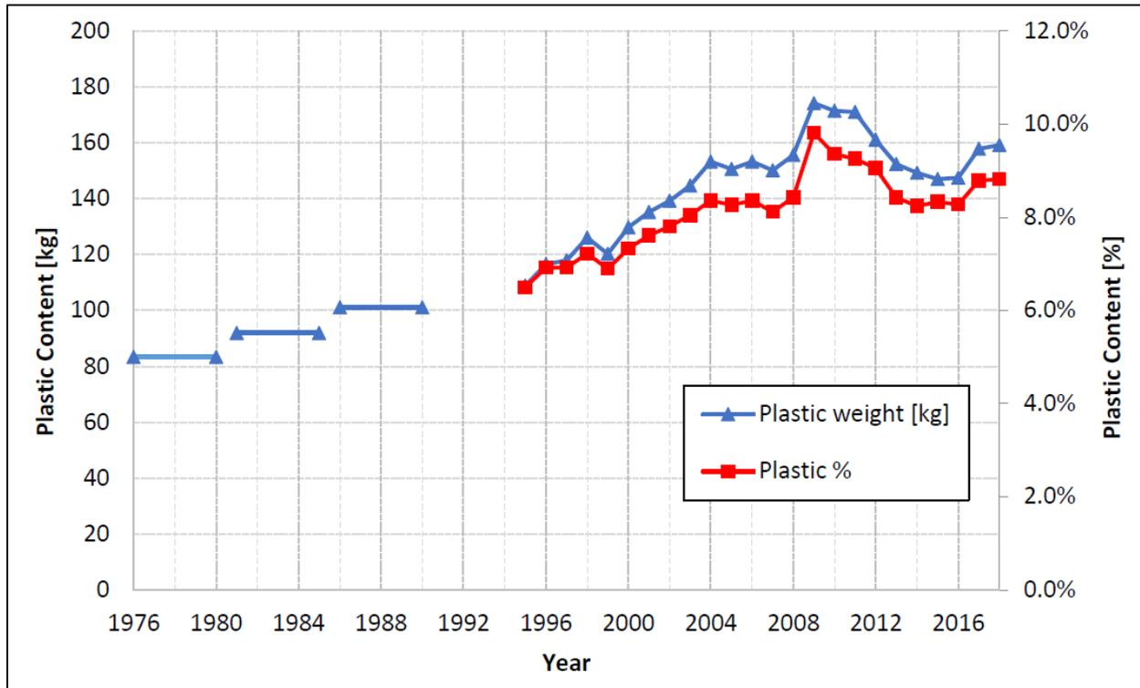
Figure 7. Plastic weight and plastic percentage of vehicle curb weight as a function of time (Figure 2 from [1]).
