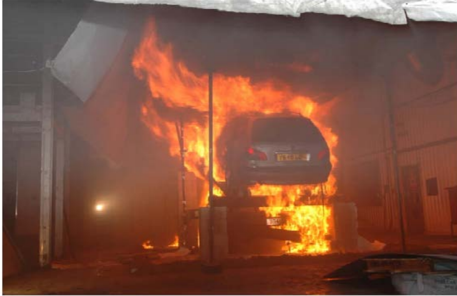
Figure 17 – Non-sprinklered test at 10 min [BRE, 2010].
