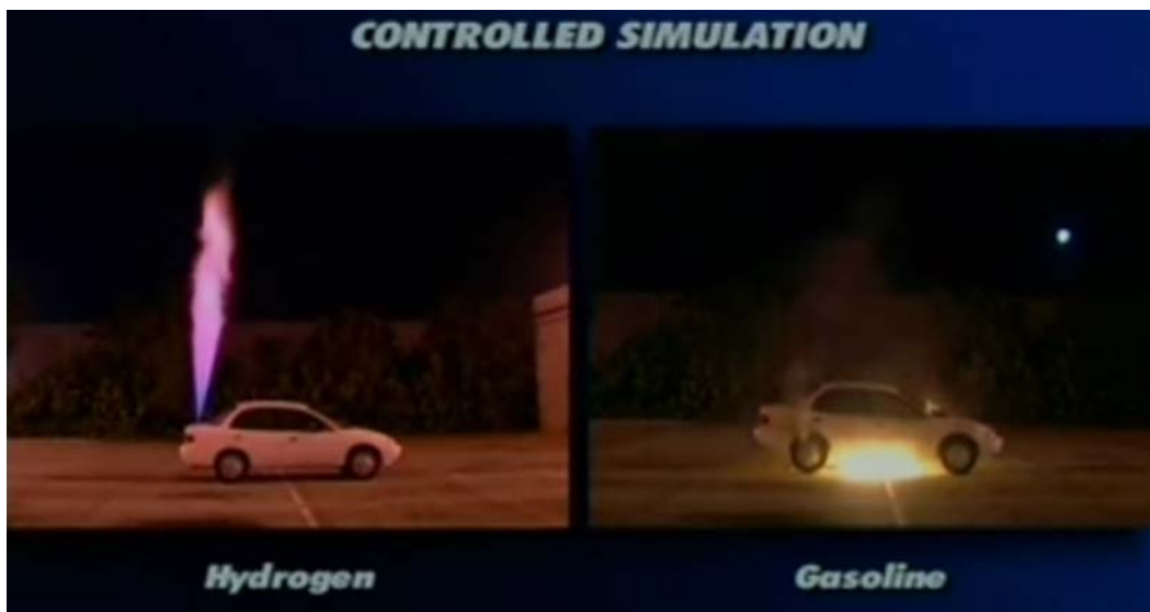
Figure 3 – Test demonstrating the difference between hydrogen and gasoline fires.
