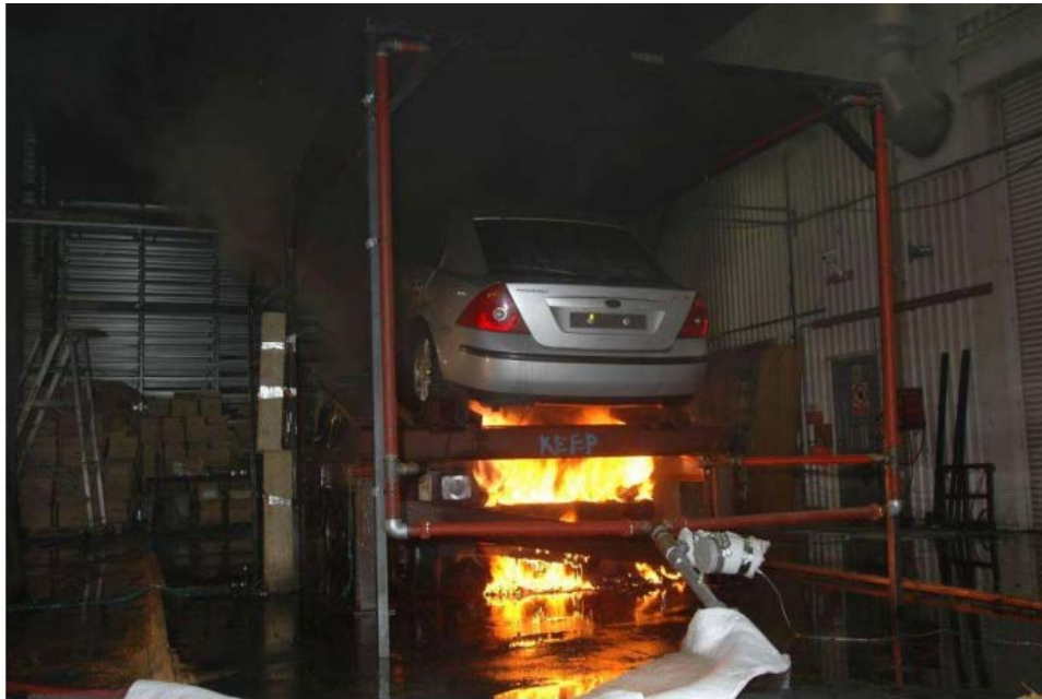
Figure 18 - Sprinklered test at 1 hour, 23 min [BRE, 2009].
