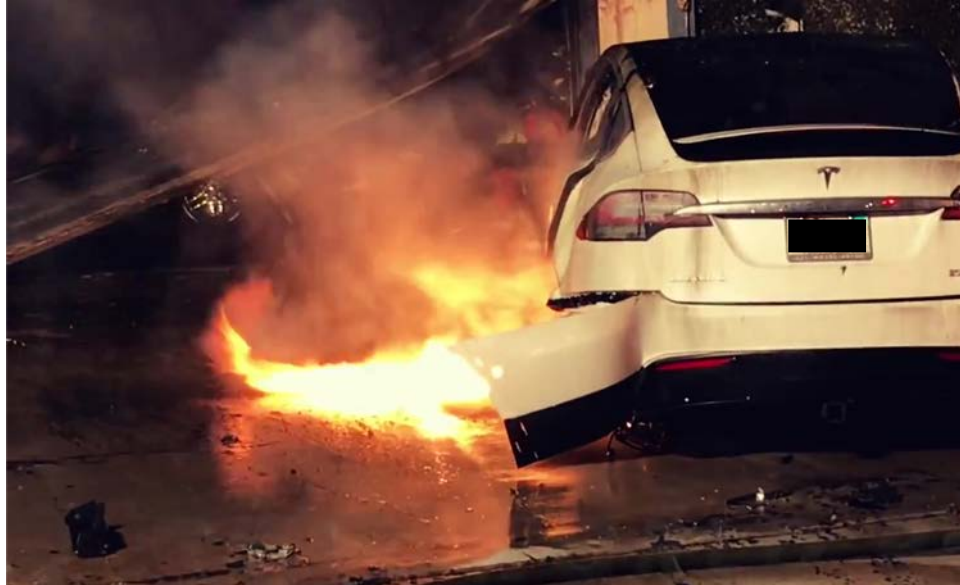
Figure 13 – Flame jet from Tesla model X battery electric car [NBC LA, 2017].
