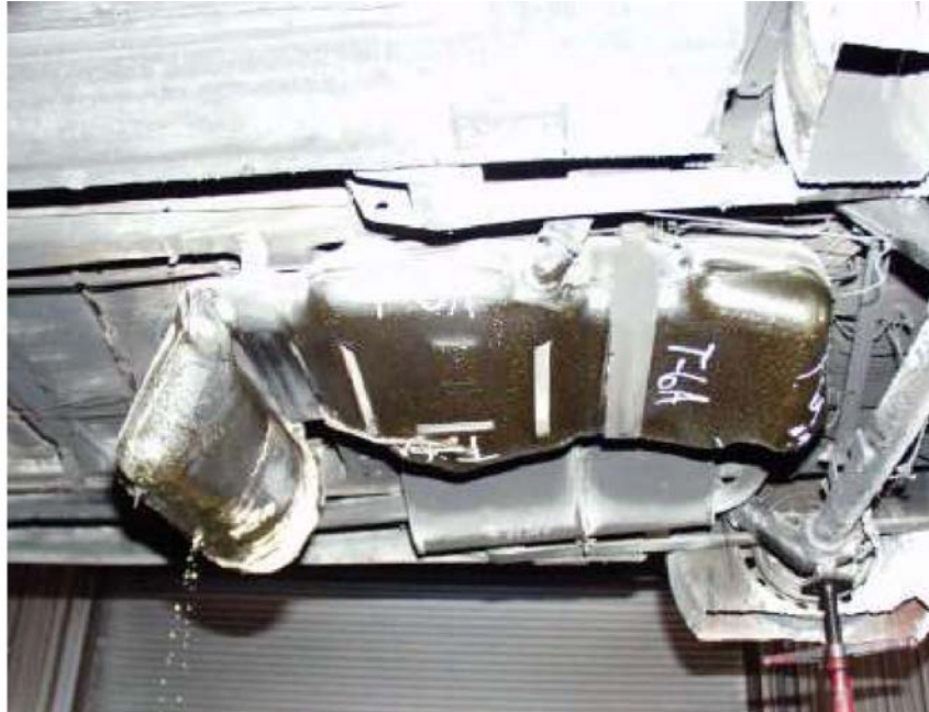
Figure 10 – Failing plastic fuel tank [Digges, 2003].
