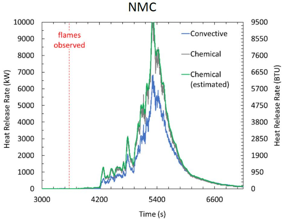
Figure 9. NMC full-scale free burn HRR. Courtesy of FM Global.
