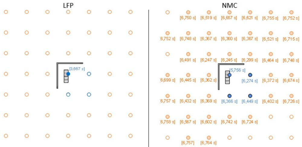
Sprinkler operation overview for LFP (left) and NMC (right) tests. Sprinklers that operated are shown as solid circles. Blue circles represent active sprinklers that could discharge water and orange circles represent indicator sprinklers that could not.
