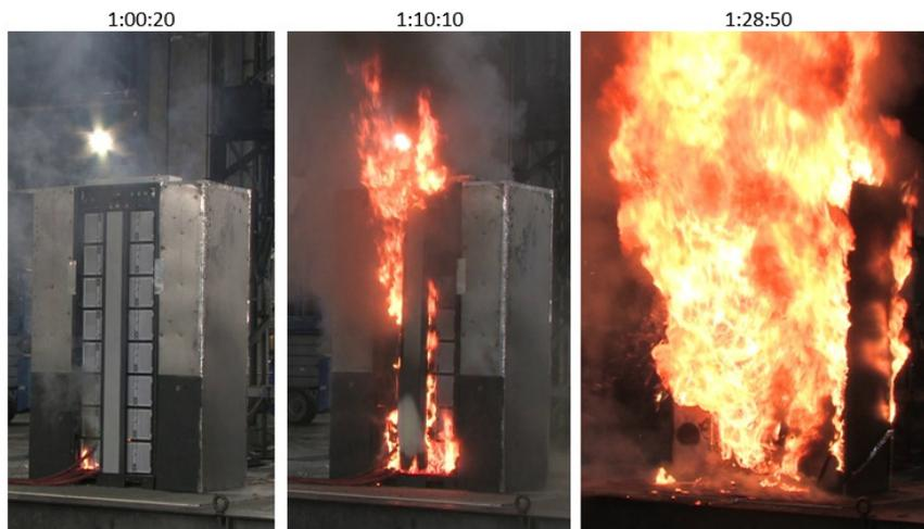
Photos of NMC fire development during large-scale free burn test: near time of ignition (left), near time of predicted sprinkler operation (middle), peak heat release rate (right).
