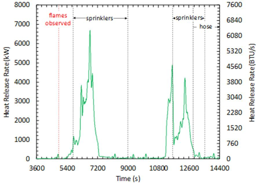
Figure 15. NMC large-scale sprinklered test HRR curve. Courtesy of FM Global.
