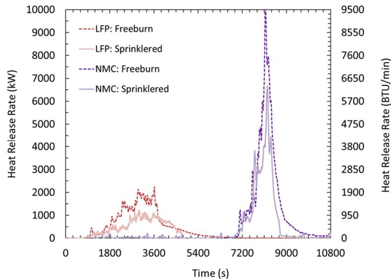
Figure 17. LFP and NMC free burn and sprinklered HRR comparison. Courtesy of FM Global.
