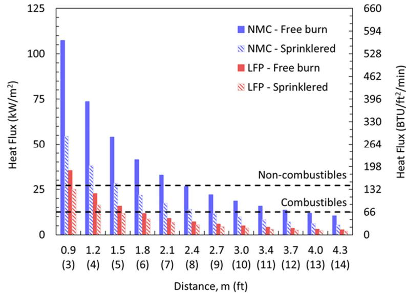
Figure 18. LFP and NMC free burn and sprinklered threshold comparison. Courtesy of FM Global.
