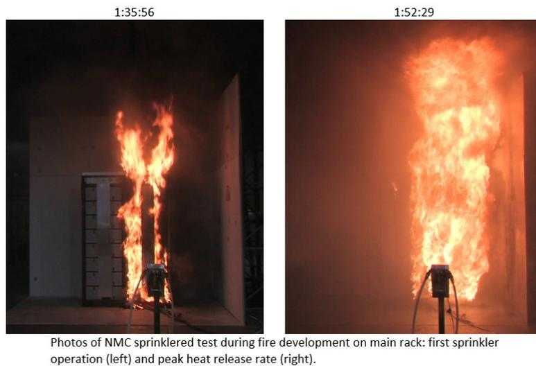
Figure 13. NMC fire development during large-scale sprinklered test. Courtesy of FM Global.
