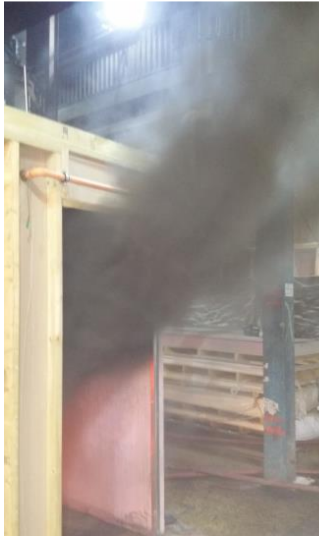
Figure 22 – Thick smoke coming out from the compartment before sprinkler activation, Experiment #2
