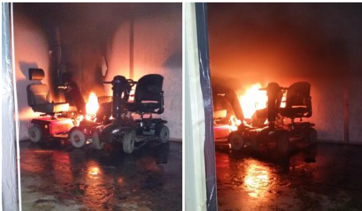
Figure 21 – Ignition of a mobility scooter in Experiment #2 (Left: immediately after ignition, right: approximately 2 minutes after ignition)
