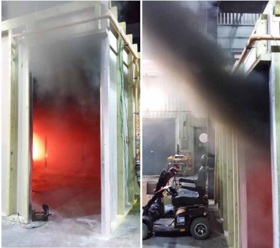
Figure 13 – Black smoke coming out from compartment, Experiment #1 (Left: front view, right: side view)
