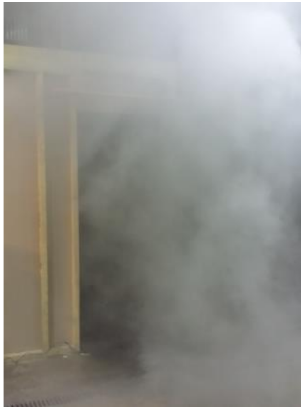
Figure 15 – Thick smoke coming out from the compartment after sprinkler activation, Experiment #1
