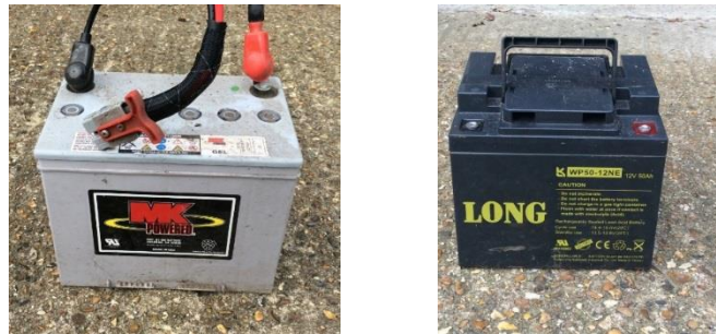
Figure 4 – Lead-acid batteries installed in the scooters.
