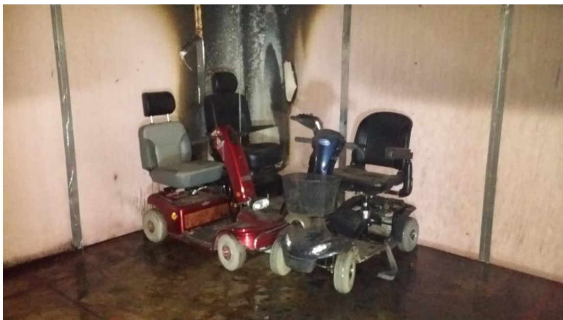
Figure 9 – Photo of mobility scooters located at the corner of the compartment, Experiment #2 (Note damage to the compartment from Experiment #1)
