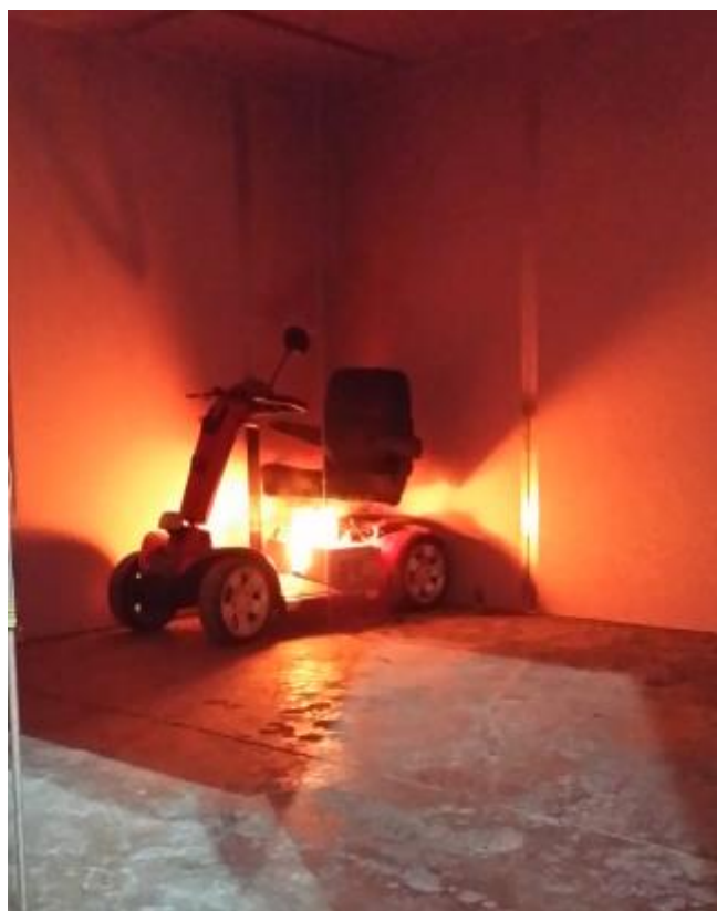
Figure 12 – Ignition of a mobility scooter in Experiment #1
