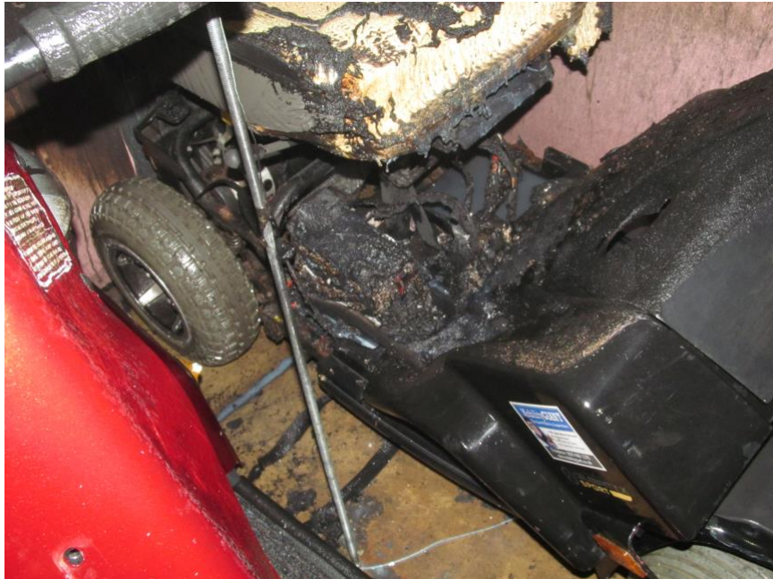
Figure 27 – Photo showing damage on mobility scooter around Li-Ion battery after Experiment #2
