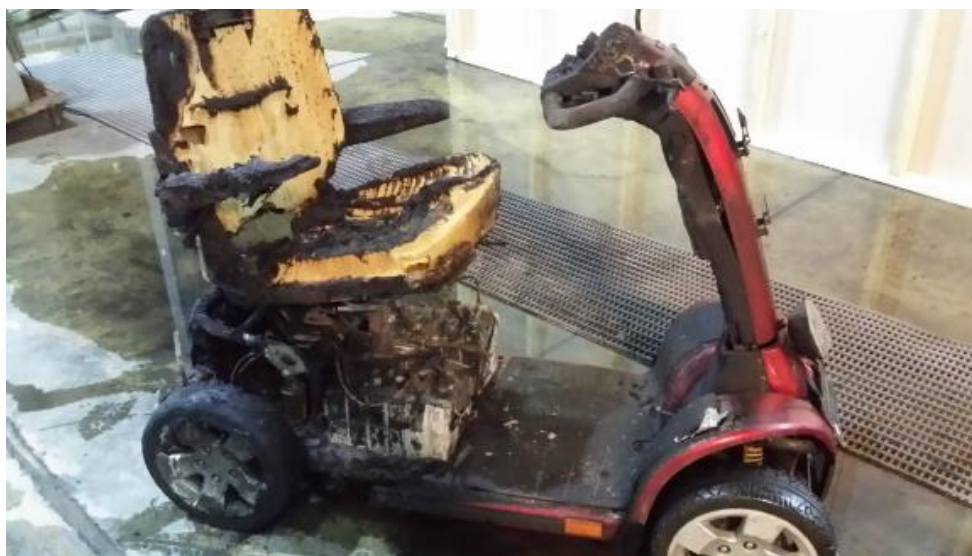
Figure 20 – Photo showing damage to mobility scooter after Experiment #1
