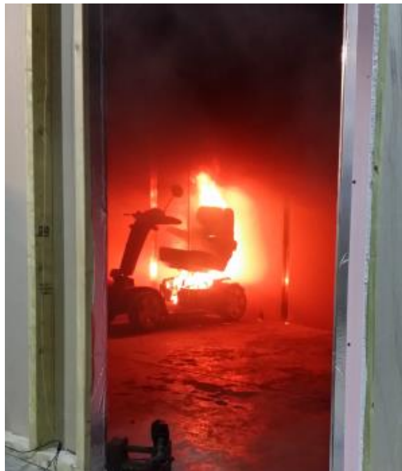
Figure 14 – Flame spread to mobility scooter seat, Experiment #1
